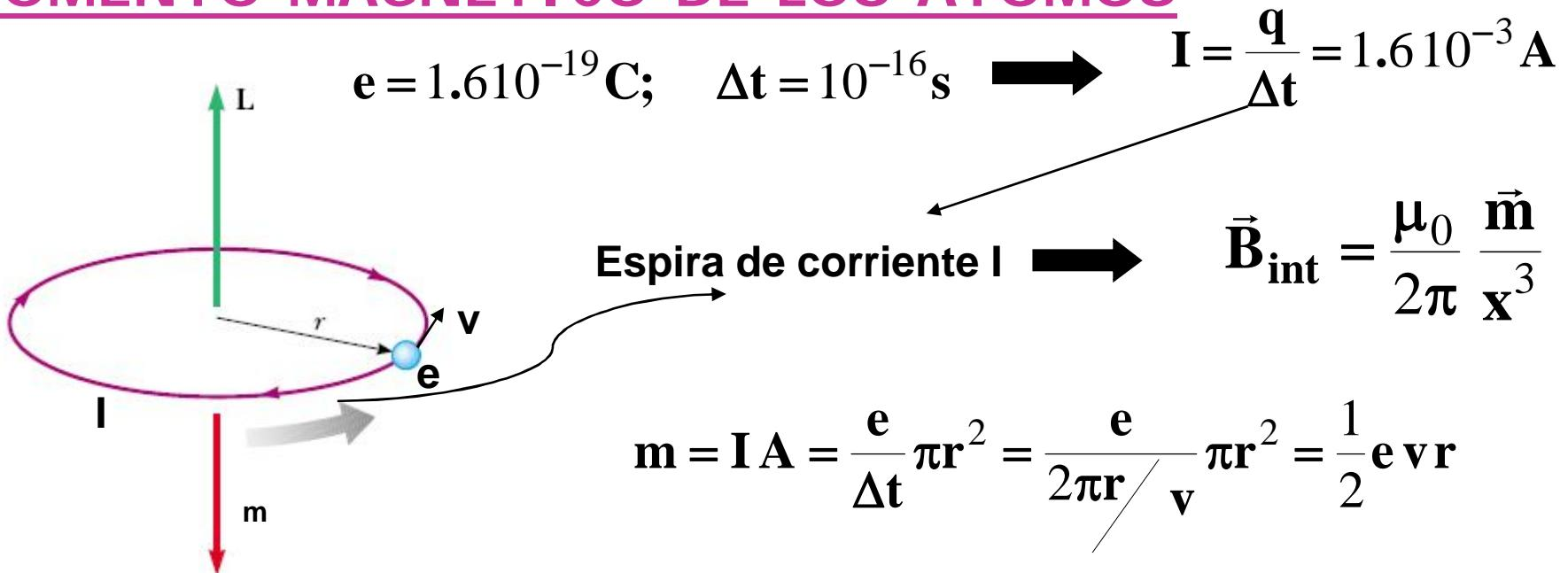
$$\text{momento angular orbital} = L = \vec{r} \times m \vec{v} = m_e v r = N \frac{h}{2\pi} \quad N \in \mathbb{Z}$$
